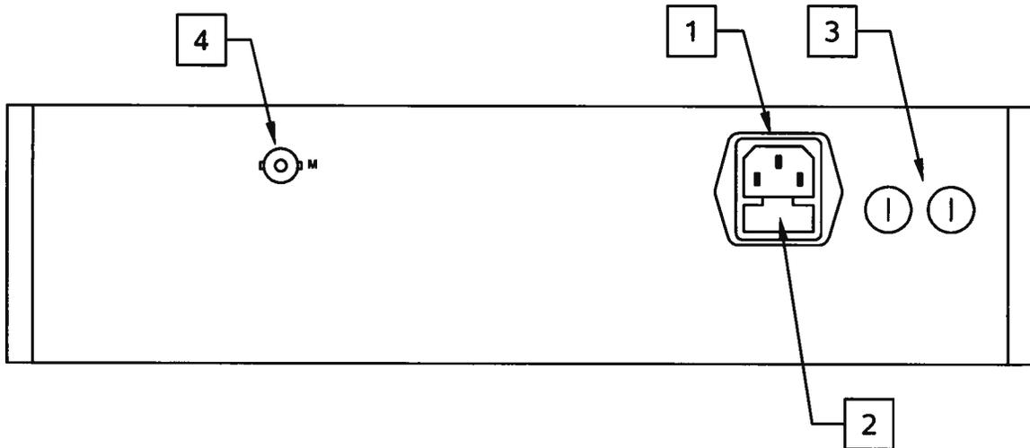
1. AC POWER INPUT. An IEC-320 C14 three-pronged recessed male socket is provided on the back panel for AC power connection to the instrument. One end of the detachable power cord that is supplied with the instrument plugs into this socket.
