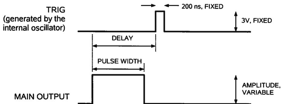
When triggered externally, the TRIG connector acts as an input. In the EXT A mode, the output parameters (pulse width, delay, and amplitude) are determined by the front panel settings. This is illustrated below:
