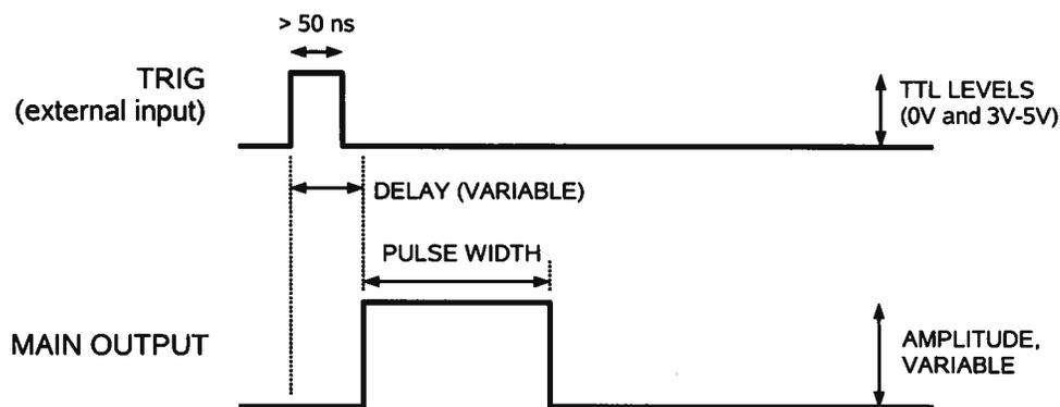
In the "EXT B" mode the instrument is triggered by a TTL-level pulse on the TRIG connector. The output pulse occurs with nominally zero delay, and the output pulse width is approximately equal to the input pulse width. The amplitude is controlled by the front panel settings. This is illustrated below:
