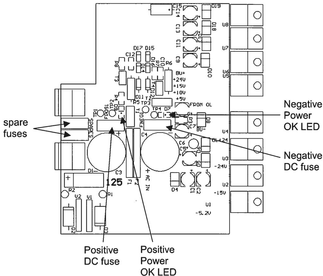
The positive fuse and one of the spare fuses on this circuit board are 2A slow-blow fuses, Littlefuse part number R452002. (This fuse can be ordered from Digikey, [www.digikey.com](http://www.digikey.com). The Digikey part number is F1345CT-ND). The negative fuse and the second spare fuse are 0.5A slow-blow fuses (Littlefuse R452.500, Digikey part number F1341CT-ND).
