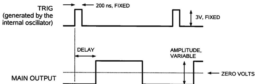
When triggered externally, the TRIG connector acts as an input. The positive duty cycle is equal to the duty cycle of the input trigger (that is, when the input trigger is logic-high, the output is positive, and when the input trigger is logic-low, the output is negative). This illustrated below:
