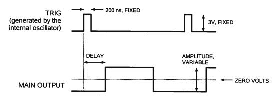
When triggered externally, the TRIG connector acts as an input. The positive duty cycle is equal to the duty cycle of the input trigger (that is, when the input trigger is logic-high, the output is positive, and when the input trigger is logic-low, the output is negative). This illustrated below:
