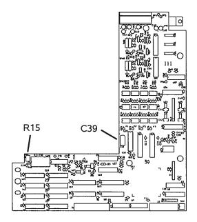
To calibrate the fine section, observe the different delays when you switch between settings of 199.0 ns and 200.0 ns. The difference between the two measurements should be 1.0 ns. If it is not, remove the top cover and locate the variable capacitor C39 on the appropriate circuit board (see the diagram below). Using a small slot screwdriver, rotate the brass screw on the capacitor until a delay increment of 1.0 ns is obtained.
