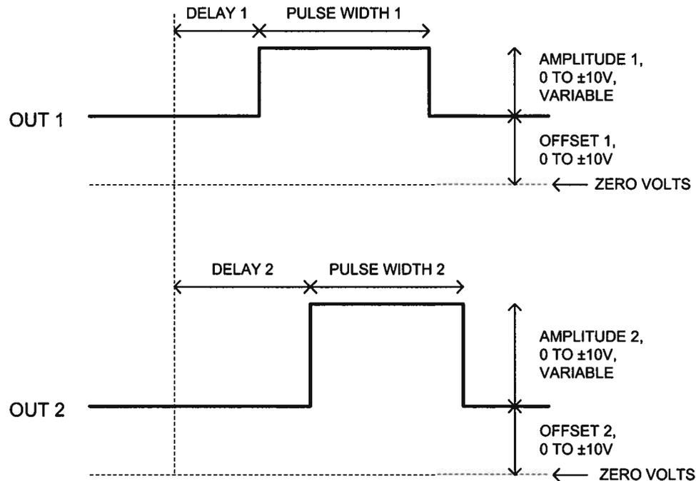
*The pulse repetition frequency is controlled by the front panel settings (or by programming commands). OUT 1 and OUT 2 trigger at the same frequency.*
