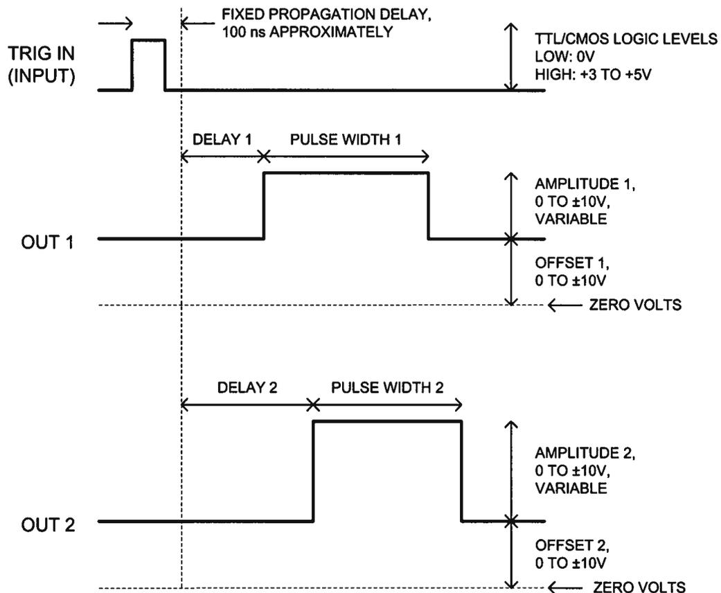
The outputs will drive load impedances as low as 50Ω.
