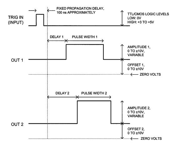
The outputs will drive load impedances as low as  $50\Omega$ .
