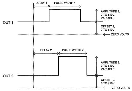
The pulse repetition frequency is controlled by the front panel settings (or by programming comands). OUT 1 and OUT 2 trigger at the same frequency.
