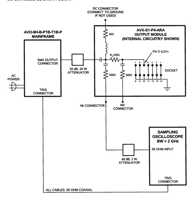
The 20 dB, 20 W attenuator included with the AVX-S1-P4-ARA should be installed between the AVO-9H-B-P1B-T1B-P mainframe and the output module, as shown
