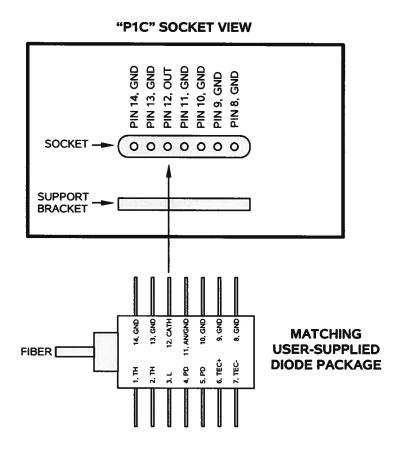
An example of a diode with the appropriate pinout is the Agere D2304G laser diode.
