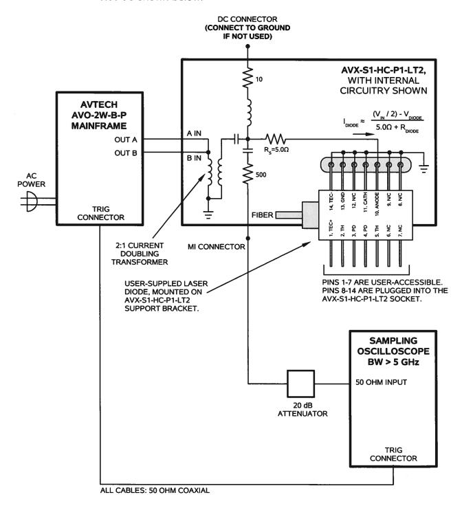
The diode load is inserted into the socket on the output module, as shown above.
