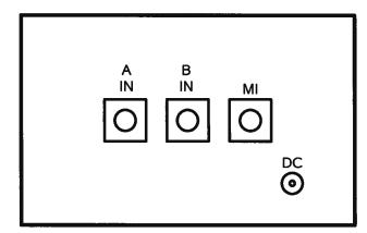
**AVX-S1-HC-P1-LT2 OUTPUT MODULE, CONNECTOR VIEW**
