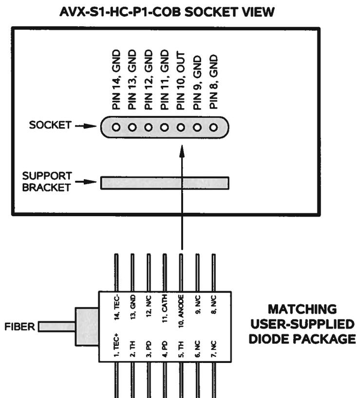
The diode series resistance must be 6 Ohms for proper operation.
