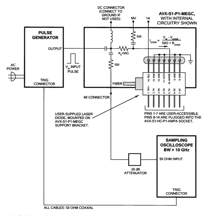
The diode load is inserted into the socket on the output module, as shown above.
