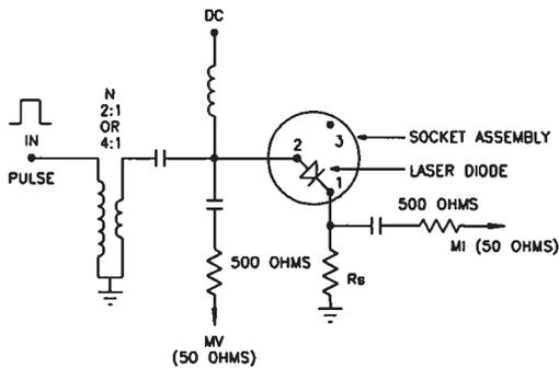
Fig. 3 - AVX-S3 functional equivalent circuit
