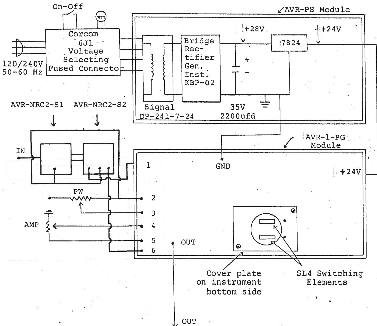
1) The AVR unit consists of five basic components or modules:
