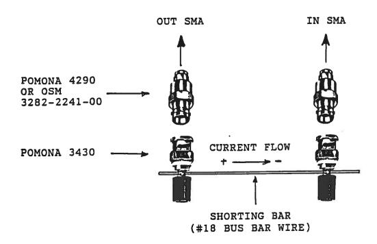
Fig. 2: SHORTING BAR, ADAPTER ARRANGEMENT FOR CURRENT PROBE
