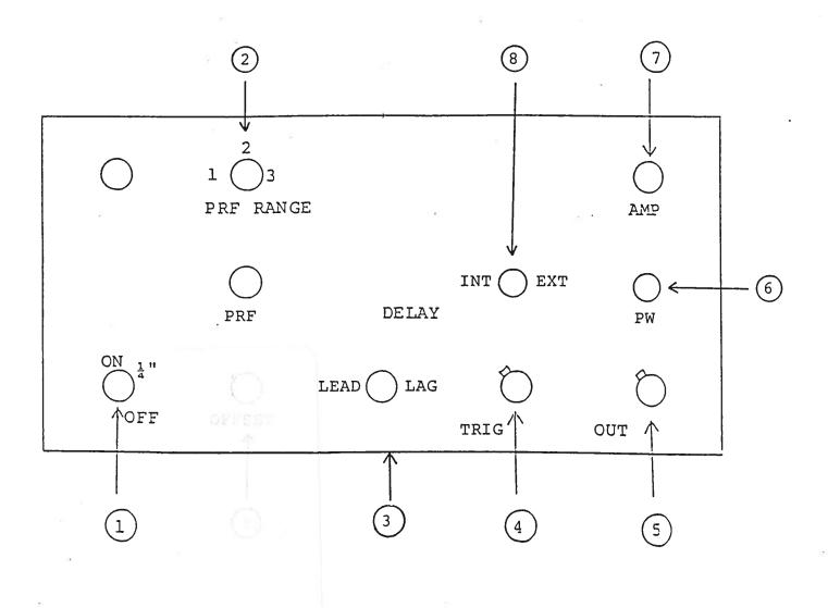
(1) ON-OFF Switch. Applies basic prime power to all stages.
