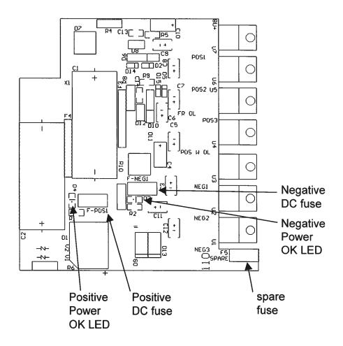
The positive fuse and the spare fuse on this circuit board are 1A slow-blow fuses, Littlefuse part number R452001. (This fuse can be ordered from Digikey, www.digikey.com. The Digikey part number is F1343CT-ND). The negative fuse is a 0.5A slow-blow fuse (Littlefuse R452.500, Digikey part number F1341CT-ND).
