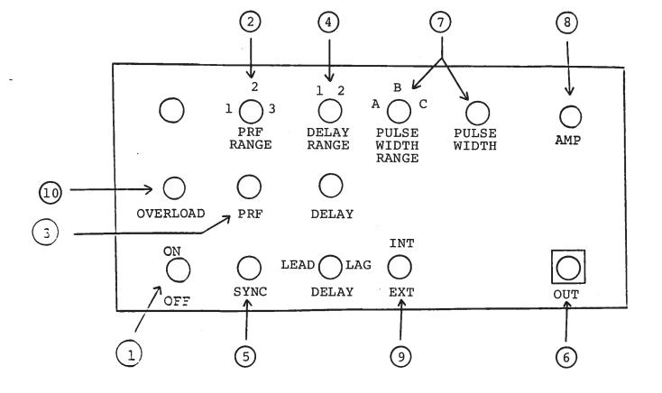
(1) ON-OFF Switch. Applies basic prime power to all stages.
