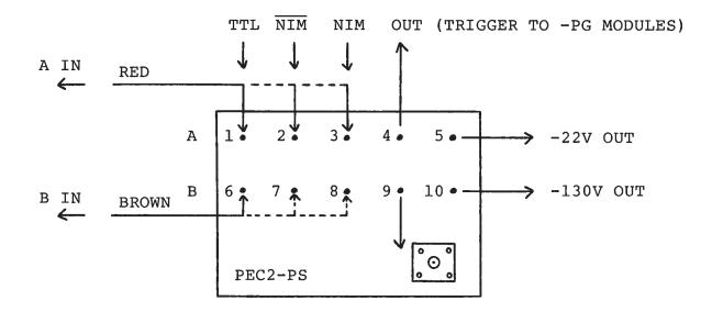
Fig. 3: PEC2-PS MODULE CONNECTIONS FOR TTL, NIM AND NIM TRIGGERING
