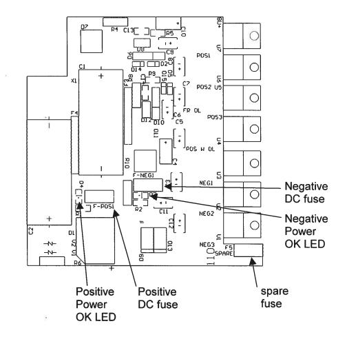
The positive fuse and the spare fuse on this circuit board are 1A slow-blow fuses, Littlefuse part number R452001. (This fuse can be ordered from Digikey, www.digikey.com. The Digikey part number is F1343CT-ND). The negative fuse is a 0.5A slow-blow fuse (Littlefuse R452.500, Digikey part number F1341CT-ND).
