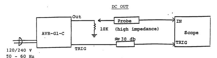
If the DC offset is employed, the "average" load resistance must exceed 10K.
