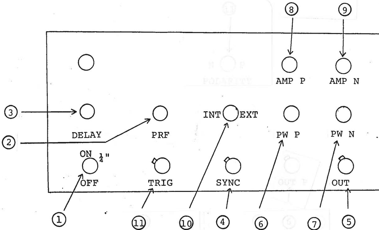
① ON-OFF Switch. Applies basic prime power to all stages.
