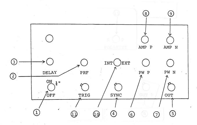
(1) ON-OFF Switch. Applies basic prime power to all stages.
