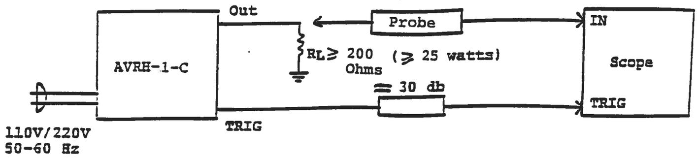
FIG. 1: PULSE GENERATOR TEST ARRANGEMENT
