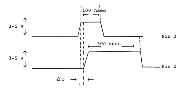
As the PW pot is varied over its full range  $\Delta T$  should vary from about 0 to approximately 100 nsec. If the waveforms at pins 2 and 3 do not resemble the above, then the -T module is defective and should be replaced. If the waveforms do resemble the above then the -PG module is at fault and should be replaced.
