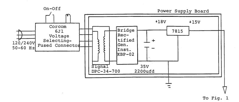
Fig. 1 System Block Diagram With Wiring And Pin Connections
