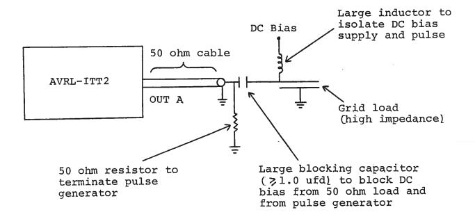
6) Output B is designed to operate directly into a high impedance load (1 K or higher). WARNING: Output B may fail if operated into a 50 ohm load (contact factory if B required to drive 50 ohm). The following arrangement is recommended when the B output is used to pulse a biased high impedance load:
