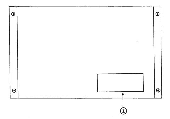
(1) <u>FUSED CONNECTOR, VOLTAGE SELECTOR</u>. The detachable power cord is connected at this point. In addition, the removable cord is adjusted to select the desired input operating voltage. The unit also contains the main power fuse.
