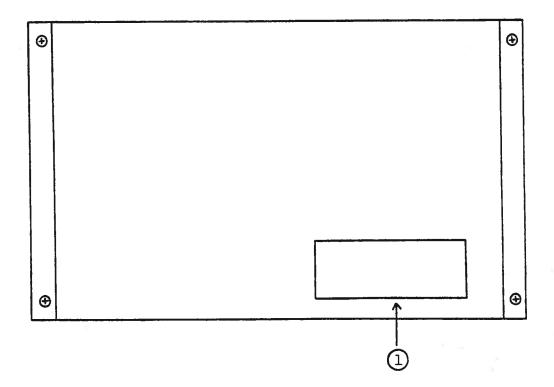
(1) FUSED CONNECTOR, VOLTAGE SELECTOR. The detachable power cord is connected at this point. In addition, the removable cord is adjusted to select the desired input operating voltage. The unit also contains the main power fuse.
