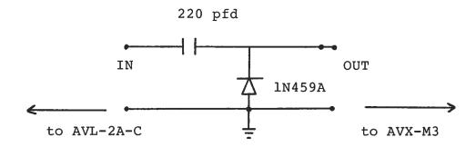
The AVS-UTA consists of a capacitor and a clipping diode which serve to introduce the large fall time to the output of the AVL-2A-C.
