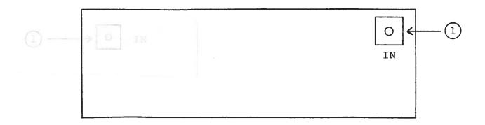
(1) <u>IN</u>. SMA connector, fifty ohm input impedance to which signal to be sampled is applied. Max input <u>+</u>1 volt.
