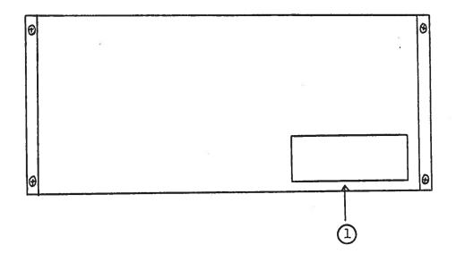
1 FUSED CONNECTOR, VOLTAGE SELECTOR. The detachable power cord is connected at this point. In addition, the removable cord is adjusted to select the desired input operating voltage. The unit also contains the main power fuse.
