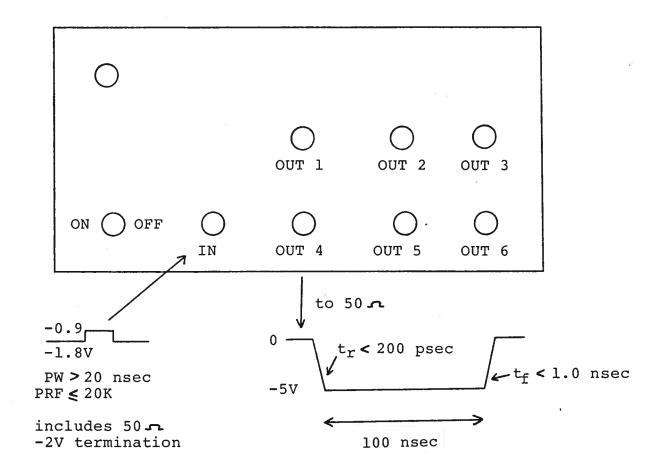
Output delayed with respect to input by \( \frac{2}{2} \) to 22.56 nsec (10 psec per bit)
