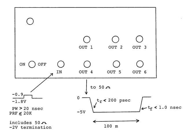
Output delayed with respect to input by≈20 to 22.56 nsec (10 psec per bit)
