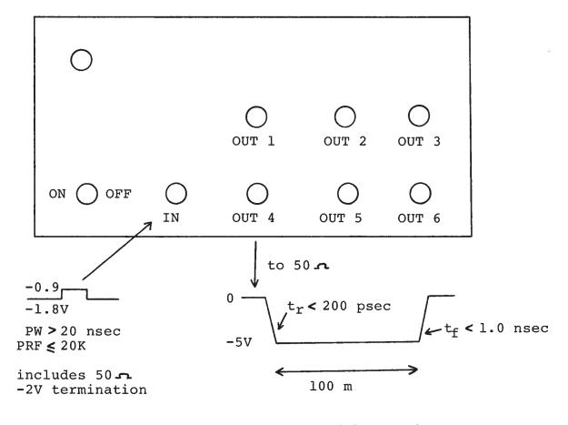
Output delayed with respect to input by ≈20 to 22.56 nsec (10 psec per bit)
