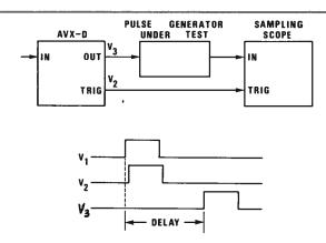
through the pulse generator under test and for the settings on the sampling scope. Model AVX-D also finds widespread application as a general purpose analog delay generator.
