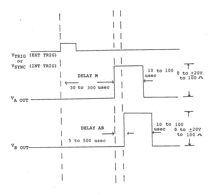
INPUT AND OUTPUT WAVEFORMS FOR AVTECH MODEL AVX-D-4-C DELAY GENERATOR
