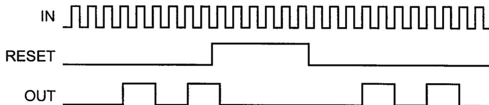
In this example,  $N=4$ . When the reset input is TTL high, the internal counter are reset to zero and are held at zero until the reset input switches to TTL low. An output pulse is generated on the fourth input pulse after the reset line returns to TTL low.
