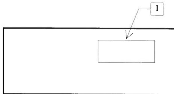
1. AC POWER INPUT. A three-pronged recessed male connector is provided on the back panel for AC power connection to the instrument. Also contained in this assembly is a 1/2A slow blow fuse and a removable card that can be removed and repositioned to switch between 120V AC in and 240V AC in.
