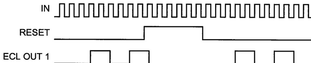
In this example,  $N=4$ . When the reset input is TTL high, the internal counter are reset to zero and are held at zero until the reset input switches to TTL low. An output pulse is generated on the fourth input pulse after the reset line returns to TTL low.
