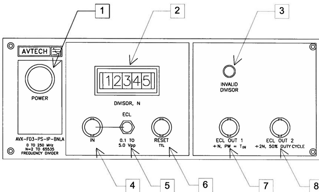
1. **POWER Switch.** The POWER push button switch applies AC prime power to the primaries of the transformer, turning the instrument on. The push button lamp (#382 type) is connected to the internal +15V DC supply.
