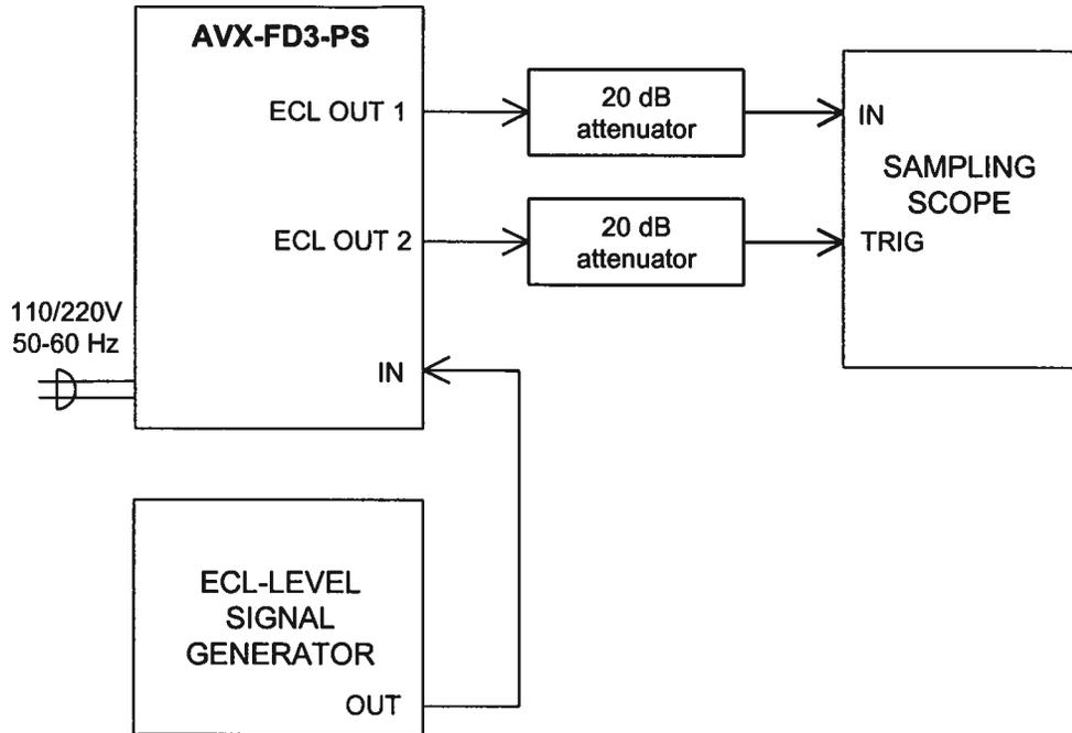
*Test Arrangement for Sampling Scopes*
