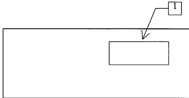
1. AC POWER INPUT. A three-pronged recessed male connector is provided on the back panel for AC power connection to the instrument. Also contained in this assembly is a 0.5A slow blow fuse and a removable card that can be removed and repositioned to switch between 120V AC in and 240V AC in.
