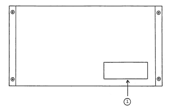
(1) FUSED CONNECTOR, VOLTAGE SELECTOR. The detachable power cord is connected at this point. In addition, the removable cord is adjusted to select the desired input operating voltage. The unit also contains the main power fuse (0.25A SB).
