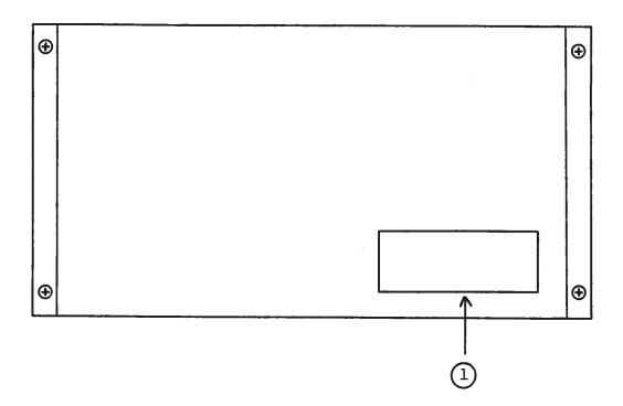
(1) FUSED CONNECTOR, VOLTAGE SELECTOR. The detachable power cord is connected at this point. In addition, the removable cord is adjusted to select the desired input operating voltage. The unit also contains the main power fuse.
