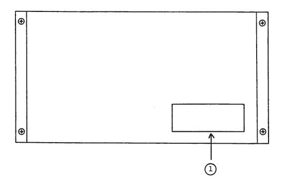
(1) <u>FUSED CONNECTOR, VOLTAGE SELECTOR</u>. The detachable power cord is connected at this point. In addition, the removable cord is adjusted to select the desired input operating voltage. The unit also contains the main power fuse (0.25 A SB).
