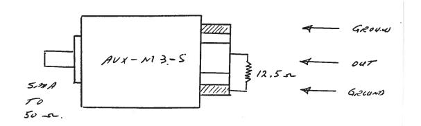
\* -SMA option: For units with the SMA option, the 12.5 Ohm load must be placed as near as possible to the OUT SMA connector.
