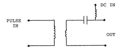
The DC bias is applied to the small solder terminal adjacent to the SMA PULSE IN connector.
