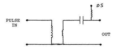
The DC bias is applied to the small solder terminal adjacent to the SMA PULSE IN connector.
