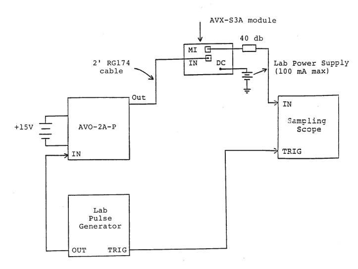
AMP: +2 to +5 Volts PRF: 0 to 20 kHz PW: >50 ns
