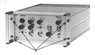
Fig. 2 Remove four 3/4" 6-32 Phillips screws
