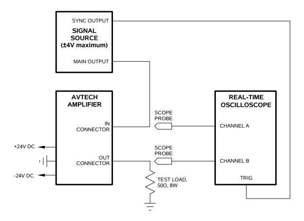
The recommended test set-up is shown above.
