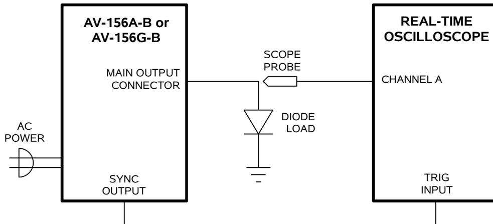
Reversing this connection may cause the diode to breakdown, possibly damaging it.
