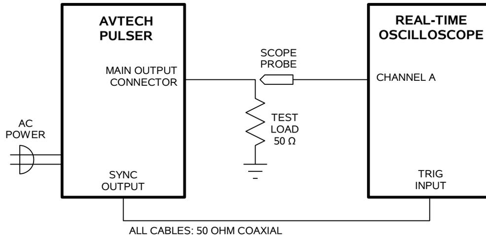
*BASIC TEST ARRANGEMENT, WITH A REAL-TIME OSCILLOSCOPE*
