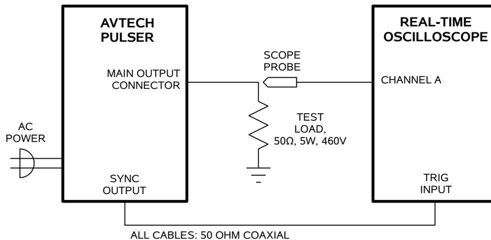
1. Connect a cable from the SYNC OUT connector to the TRIG input of an oscilloscope. Connect a 5W (or higher) 50Ω load with a voltage rating > 460V to the OUT connector and place the scope probe across this load. Set the oscilloscope to trigger externally with the vertical setting at 100 Volts/div and the horizontal setting at 50 ns/div.
